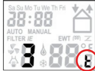
Once the programmed time delay is complete, the ComfoAir automatically switches back to the previous ventilation setting.
