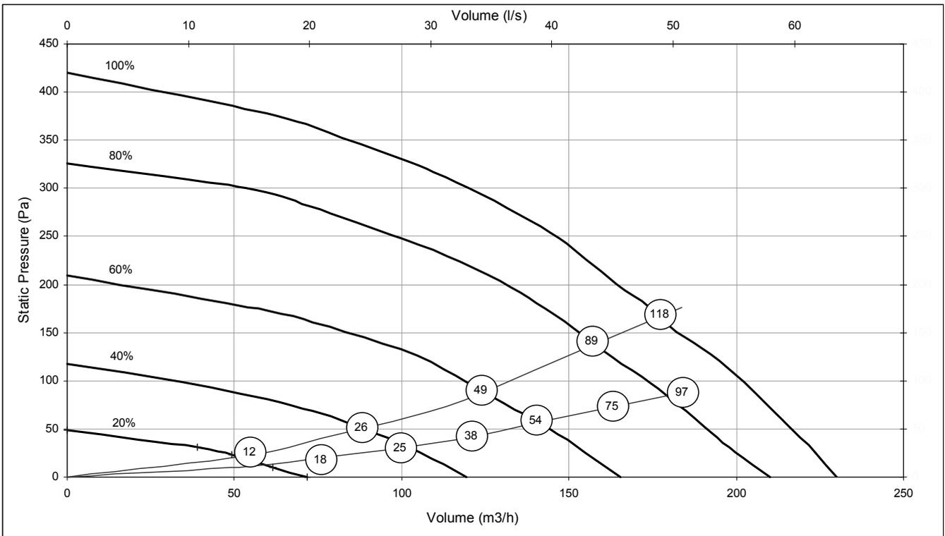
Note: Graph show 2 typical system curves with total unit input power in Watts.
