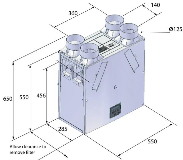
Figure 3: Sentinel Kinetic Dimensions
