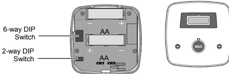
3. Ensure that the system address, set by the 6-way DIP switch on the Wireless Switch PCB matches that on the Wireless Receiver PCB. For multiple systems in close proximity to each other, the system addresses need to be different. The Wireless Switch PCBs also have a 2-way DIP switch to set the transmitter address. Up to four Wireless Switch's can be used to control any one unit. The Wireless Switch address needs to be different for each Switch in a system.
