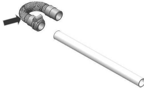
6. Fit pipe assembly into waste pipe and secure to condensate spigot with worm drive clip.
