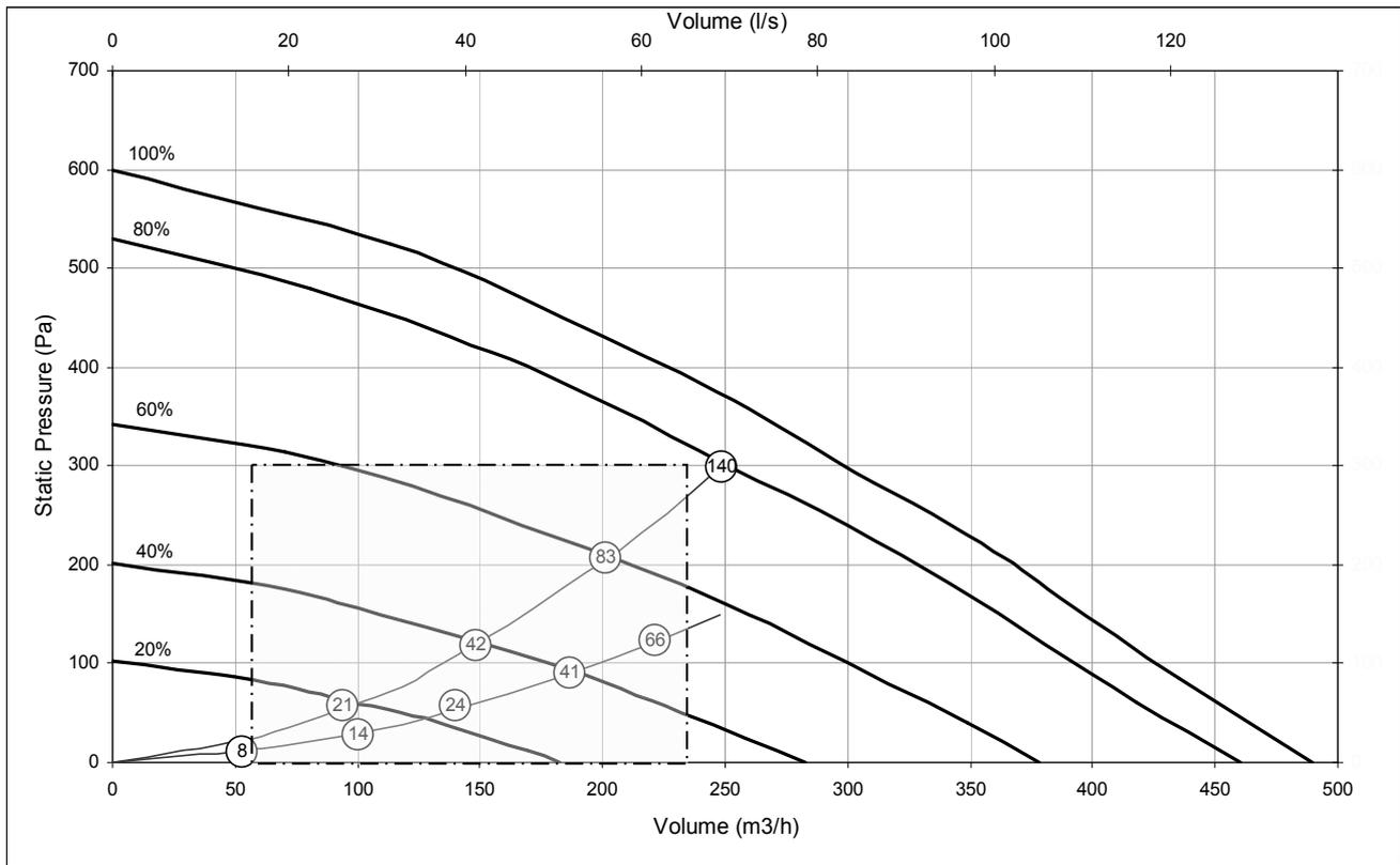
Note: Graph shows 2 typical system curves with total unit input power in Watts and the shaded area of the graph shows constant volume operation (CVP only).
