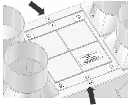
The arrow labels on the top edge of the Covers should be correctly matched to the arrow labels on the top of the Case.
