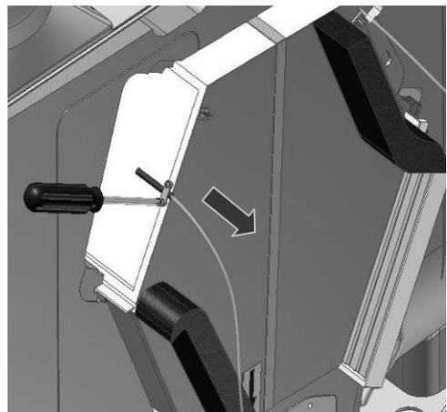
4. Pull out the cell and make sure that the rear bottom of the cell is securely resting on the lower edge of the foam so you can access the rear pressure tube. Repeat step 3 to detach the rear pressure tube. When the rear pressure tube is removed then the cell is free to clean.
