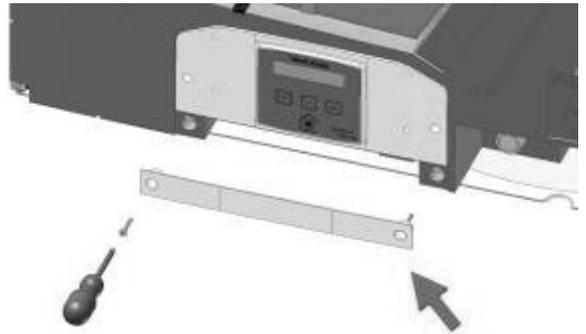
5. Remove the 2 screws and detach the Control Panel and disconnect the mains lead.
