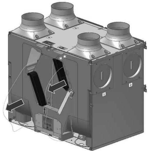
3. Pull out the Heat Exchanger Cell to gain access to the 2 screws on the cell as shown opposite. Loosen up the both screws (no need to remove them completely) to be able to remove the pressure tube and its rubber grommet strip.
