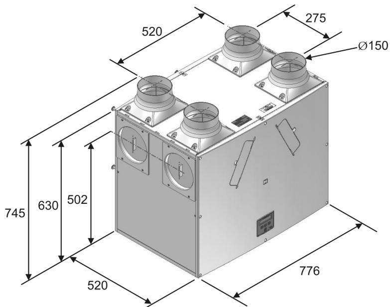
Figure 4: Sentinel Kinetic Plus Dimensions
