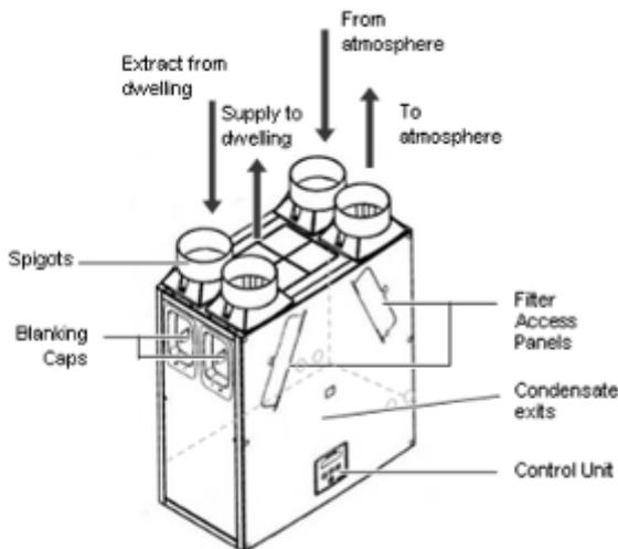
Fig 1: Sentinel Kinetic (Front of Unit as supplied)
