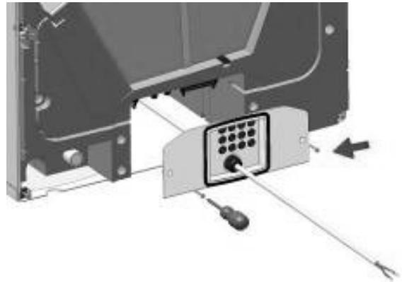
7. Re-attach the Cable Inlet Plate on the opposite side of the unit.
