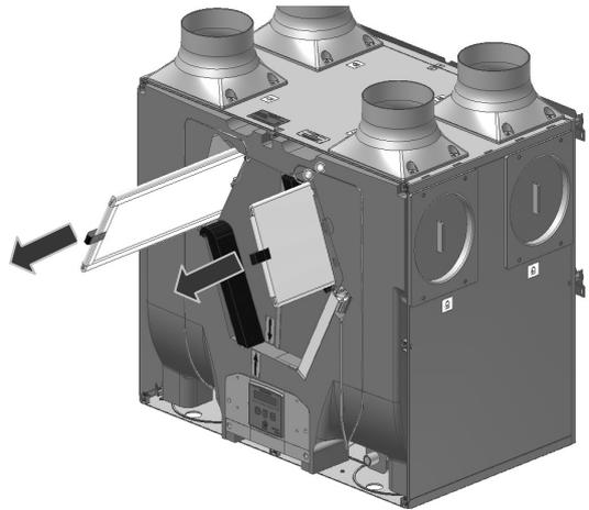
2. Remove both pressure tubes from their channels and let them remain suspended in the air as shown opposite.
