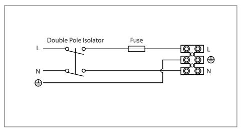
Supply wiring diagram 230V~50Hz ref EE 141
