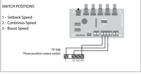
Three Position Rotary Switch TP 508 switching and connection ref EE 147
