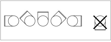
**Duct Heater fitting orientation**
